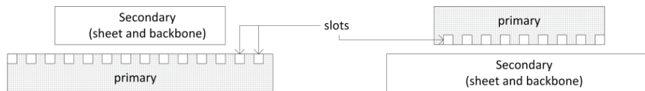
Fig. 4. Comparison short-secondary LIM (left) to short-primary LIM (right)
