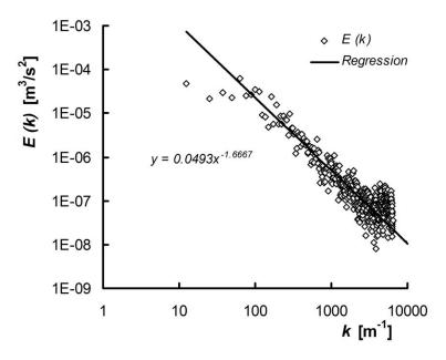
Fig. 5. Energy spectrum function – axial direction, N = 450 rpm, Van Doorn's convective velocity
