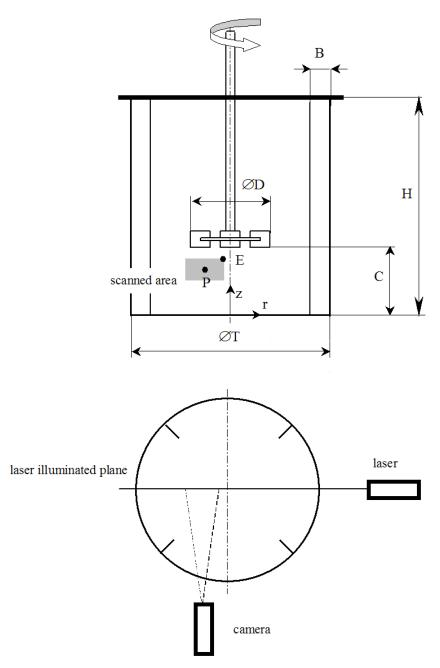
Fig. 1. Scheme of experimental apparatus and investigated area
