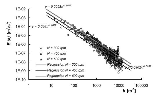
Fig. 6. Energy spectrum function – radial direction, effect of impeller speed, Van Doorn's convective velocity
