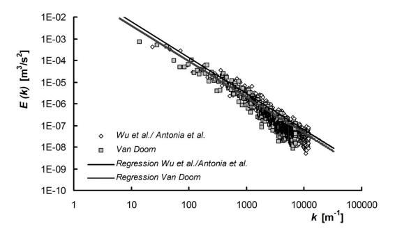
Fig. 7. Effect of convective velocity formula on energy spectrum function - radial direction, N = 600 rpm
