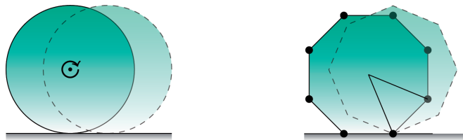
Fig. 1. A rigid ring and a rigid octagon rolling over a flat surface
