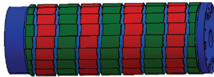
Fig. 4. Linor with skewed permanent magnets
