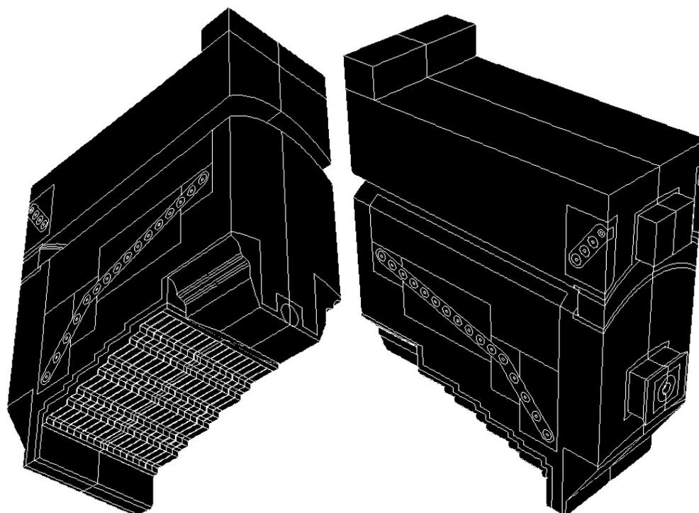
Fig. 4. Geometrical model of the boiler furnace
