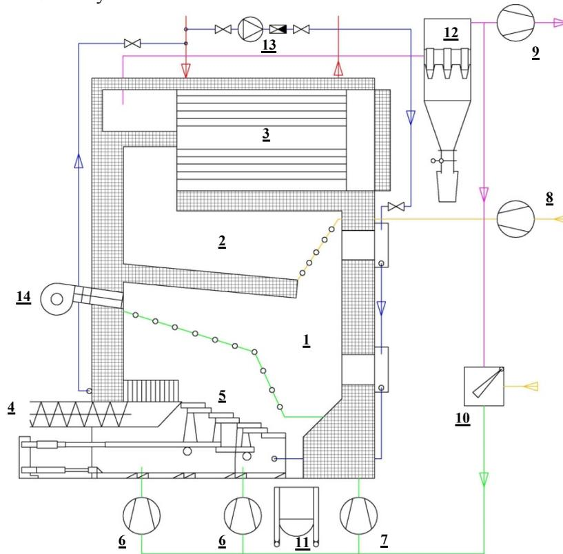
Fig. 1. Boiler flowchart;
