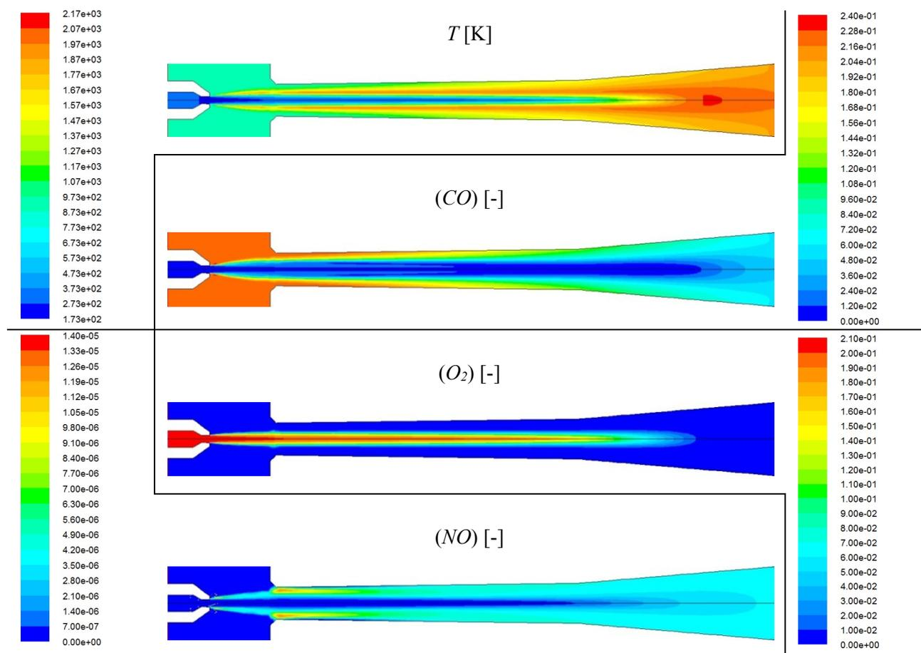
Fig. 6. Fields of temperature [K] and of the CO, O<sub>2</sub> and NO molar contents [-] in the axial section of the jet blower area
