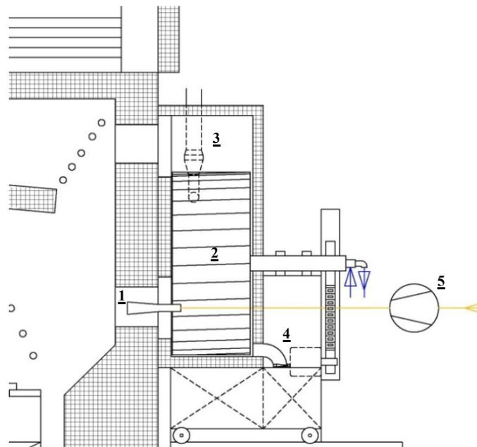
Fig. 2. Gasifier flowchart – integration with the boiler;
