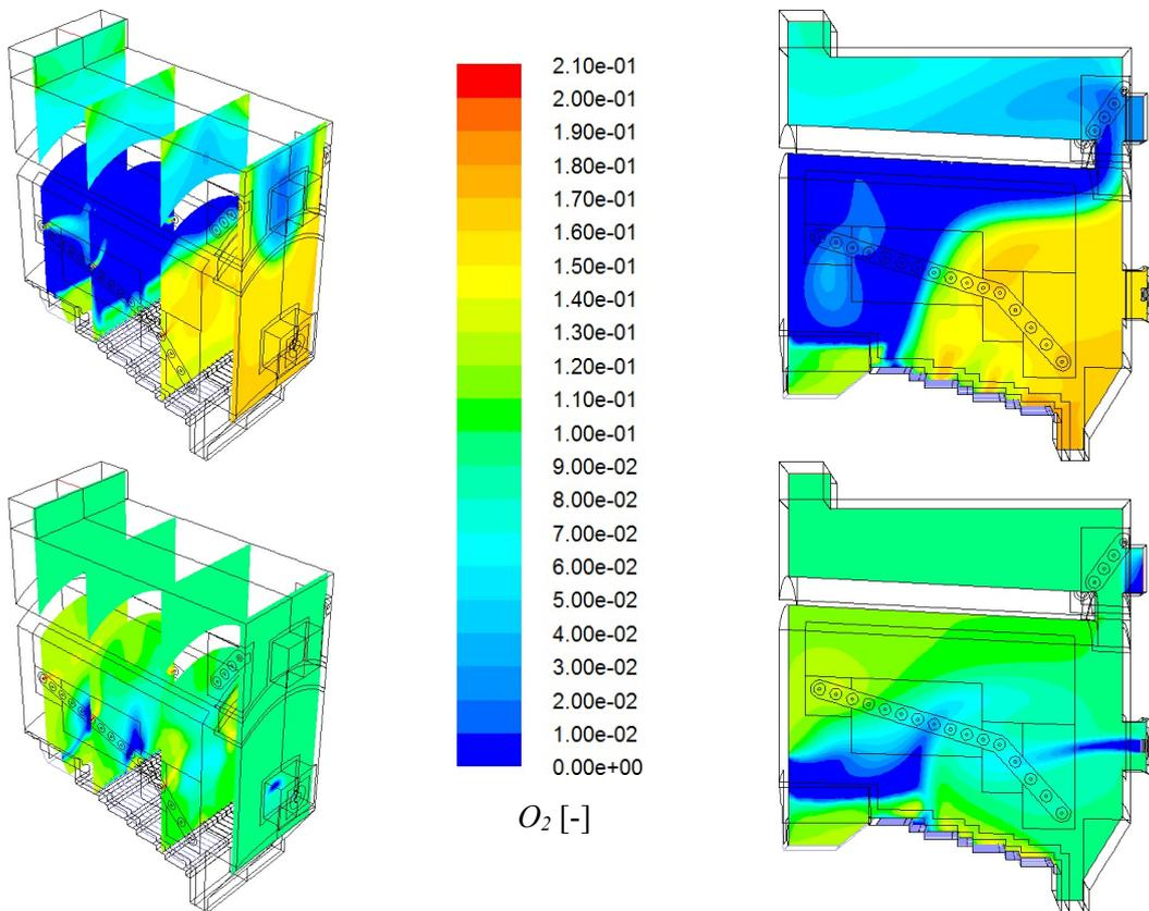
Fig. 10. O<sub>2</sub> molar content fields for the boiler in the reference state (top) and in the post-upgrade state (bottom)
