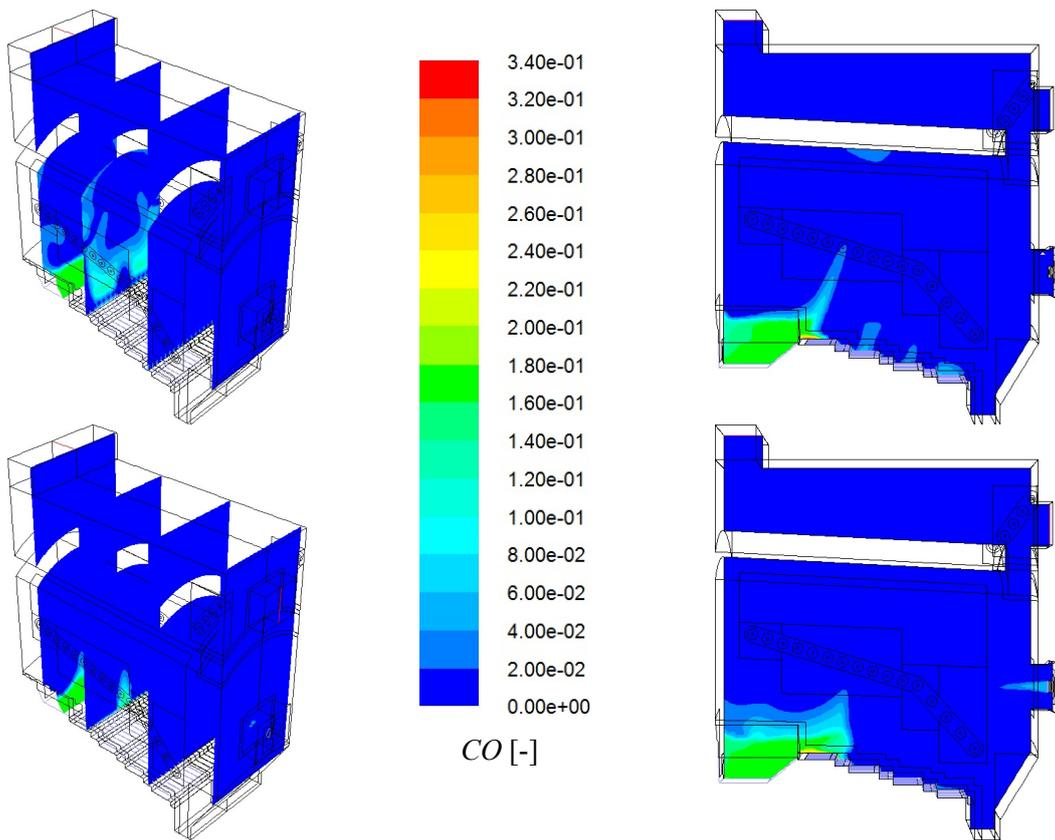
Fig. 9. CO molar content fields for the boiler in the reference state (top) and in the post-upgrade state (bottom)
