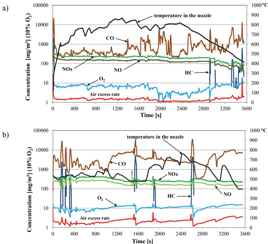
Fig. 3. Comparison of the parameter variation in time (oxygen and pollutant concentrations: CO, HC, NO, NO<sub>x</sub> in the flue gas, temperature in the nozzle, air excess ratio) between the two batches fired with (a) high combustion air flow rate and (b) low combustion air flow rate
