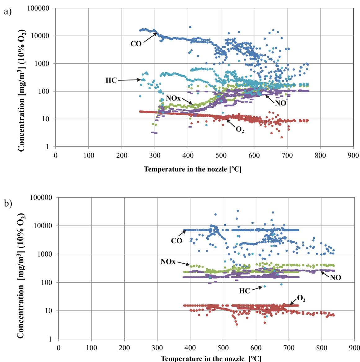
Fig. 4. Oxygen and pollutant (CO, HC, NO, NO<sub>x</sub>) concentrations in the flue gas versus temperature in the wood gas firing nozzle/combustion chamber; comparison between (a) the batch fired with high combustion air flow rate and (b) the batch fired at low combustion air flow rate
