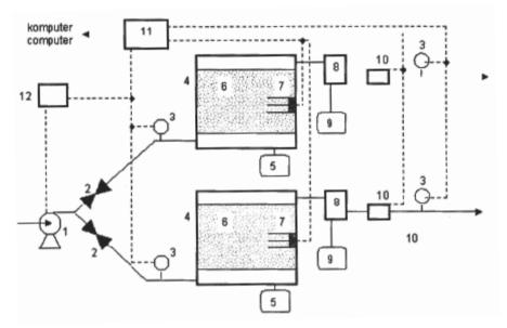
Fig. 1. Schematic diagram of the bioreactor: 1 – pump, 2 – flow regulator, 3 – flow meter, 4 – isolated chambers, 5 – drained liquides container, 6 – composted mass, 7 – sensors array, 8 – air cooling system, 9 – condensate container, 10 – multiplate gas sensor array, 11 – 32 chanel recorder, 12 – 1ir pump steering system air
