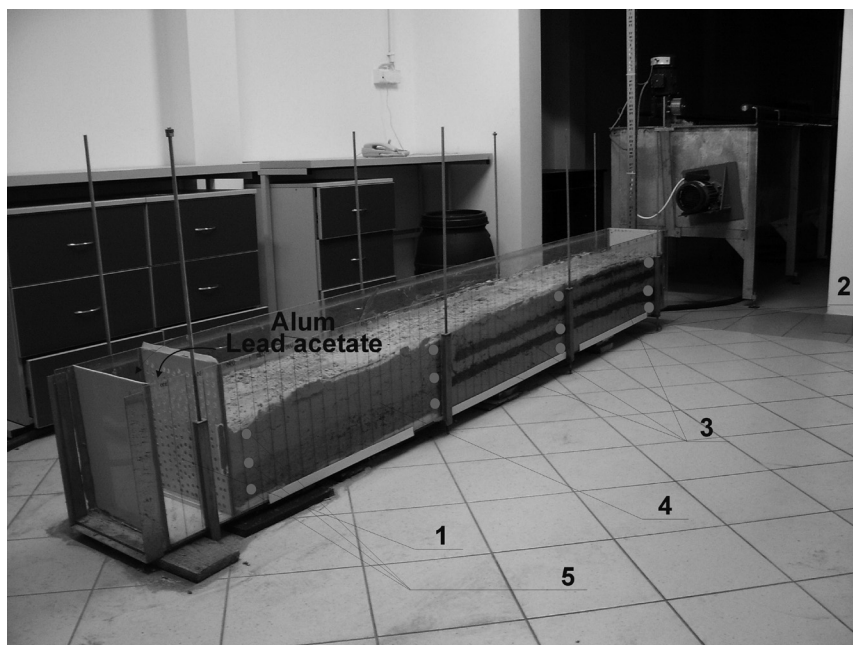
Pic. 2. Horizontal column filled with alluvial deposits. 1 – separated part of the device supplied with Cr and Pb compounds, 2 – artificial slope simulating slope of floodplain, 3 – peats, 4 – alluvial fine sands, 5 – places of samples' collection
