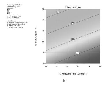
Fig. 3. 3D surface and contour plot for nickel extraction. (a) Influence of the acid concentration and solid-liquid ratio on the overall nickel extraction, (b) Influence of the acid concentration and reaction time on the overall nickel extraction, (c) Influence of the reaction time and solid-liquid ratio overall nickel extraction
