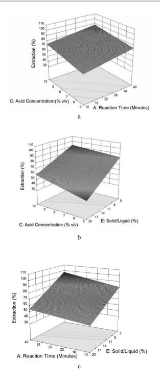
Fig. 2. The effects of Main variable interaction on the nickel extraction, a: acid concentration and reaction time, b: acid concentration and Solid/liquid ratio, c: Solid/liquid ratio and reaction time
