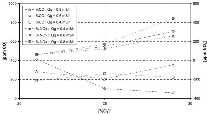
Fig. 6. Effect of oxygen concentration on CO and NO contents for different gas flows ( $\lambda=1.25$ )
