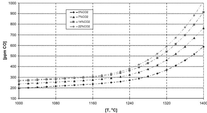
Fig. 13. Equilibrium concentration of CO depending on the temperature and CO<sub>2</sub> concentration in 25%O<sub>2</sub>/N<sub>2</sub>/CO<sub>2</sub> mixture for stoichiometric combustion
