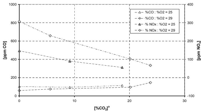
Fig. 10. Effect of CO<sub>2</sub> addition on CO and NO concentration for different O<sub>2</sub> contents ( $\lambda = 1.25$ , gas flow 0.6 m<sup>3</sup>/h)
