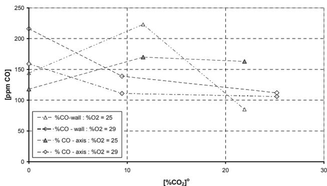
Fig. 4. Variation of CO concentration on a cross section of the chamber ( $\lambda = 1.15$ , gas flow 0.6 m<sup>3</sup>/h)
