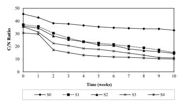
Fig. 5. Evolution of C/N ratio during the composting process
