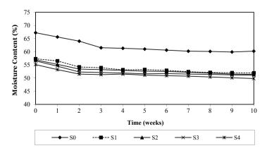
Fig. 2. Evolution of moisture content during the composting process
