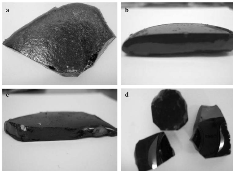
Fig. 4. The products of plasma treated wastes: **a** – ash from sewage sludge (40 g) + carbonate fraction (10 g), **b** – slag from municipal waste (40 g) + carbonate fraction (10 g), **c** – slag from medical waste (40 g) + carbonate fraction (10 g), **d** – slag from hazardous and industrial waste (40 g) + carbonate fraction (10 g)
