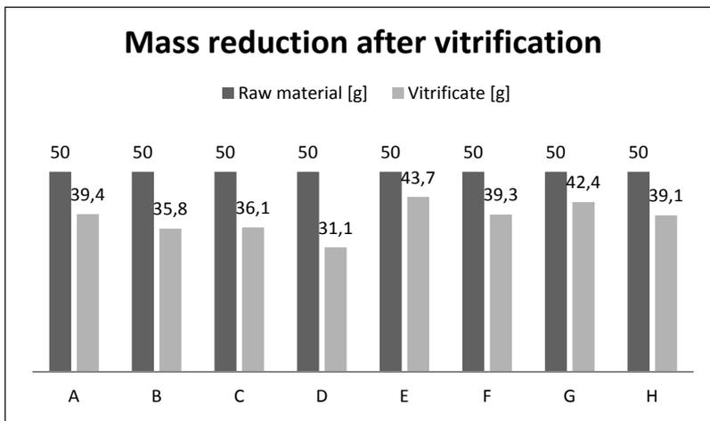
Fig. 5. Raw material mass reduction after vitrification
