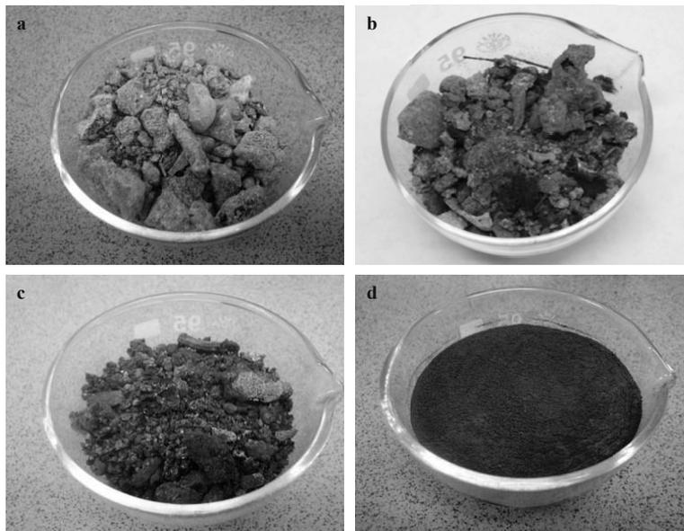
Fig. 1. Substrates: **a** – slag from municipal wastes grate furnace incineration, **b** – slag from medical waste Purotherm Pyrolyse treatment, **c** – slag from industrial and hazardous waste kiln incineration, **d** – ash from sewage sludge fluidized-bed furnace incineration
