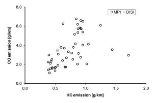
Fig. 5. A scatterplot of HC and CO emissions results for all test vehicles, tested over the UDC at -7°C
