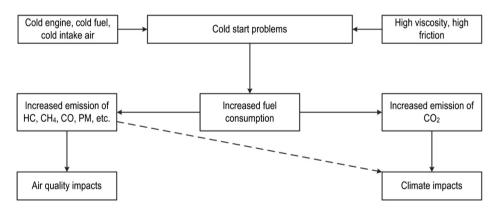
Fig. 1. Cause-and-effect diagram of the impacts of cold-start engine operation at low ambient temperatures on air quality and climate
