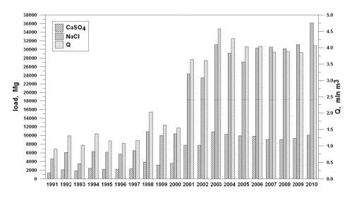
Fig. 3. Time series of chlorides and sodium loads as NaCl and sulphates and calcium as  $CaSO_4$  captured yearly by the wells barrier near the facility, and abstracted saline water (Q)
