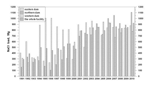
Fig. 6. Time series of NaCl load captured within a year by single well of barrier around the whole facility and in particular barrier parts along the dams
