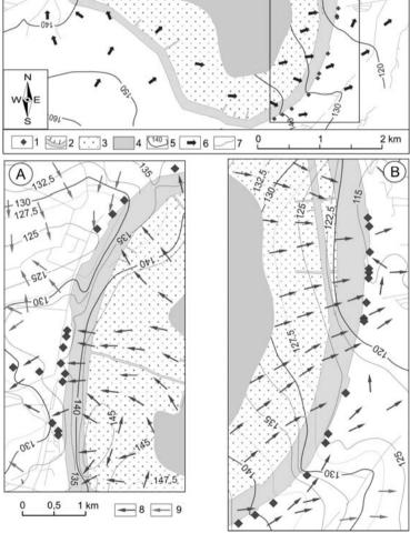
Fig. 1. Želazny Most tailings disposal site and a wells barrier: 1 – drainage well, 2 – dam, 3 – tailings,
