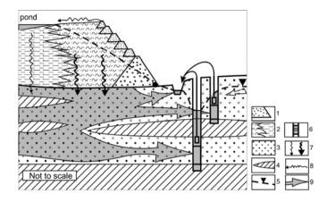
Fig. 2. Model of capturing contaminated groundwater by a drainage wells barrier (after [21], modified):
