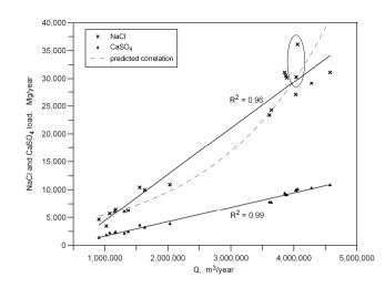
Fig. 4. Chlorides and sodium loads as NaCl and sulphates and calcium as  $CaSO_4$  captured by the wells barrier near the facility vs. abstracted saline water (Q)
