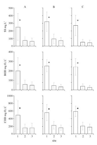
**Fig. 1.** Changes in concentration of SS,  $BOD_5$  and COD (mean  $\pm$  1SD, n= 18) on consecutive sites (1 – inlet to AP, 2 –inlet to LP, 3 – outlet from LP, \* indicated significant difference within system, P = 0,05) in three Lemna Systems (A – Falęcin Stary, B – Raków, C – Bąkowiec)
