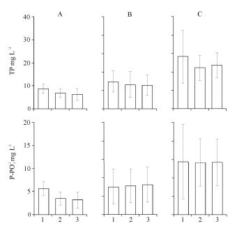
**Fig. 3.** Changes in concentration of TP and P-PO<sub>4</sub><sup>-3</sup> (mean ± 1SD, n= 18) on consecutive sites (1 – inlet to AP, 2 – inlet to LP, 3 – outlet from LP) in three Lemna Systems (A – Falęcin Stary, B – Raków, C – Bąkowiec)
