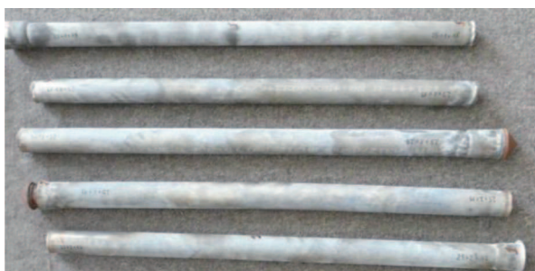
Fig. 3. Bimetallic bars after explosive welding
