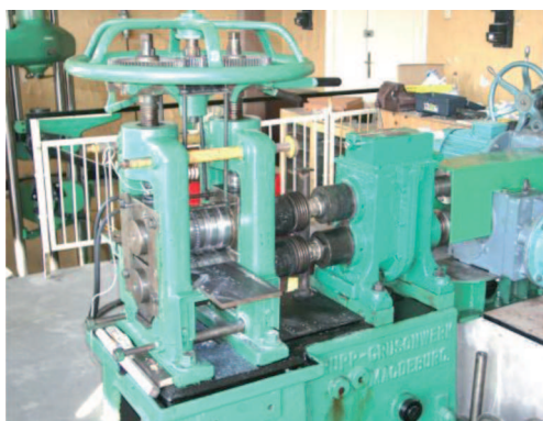
Fig. 12. Laboratory rolls Ø150 mm – general view
