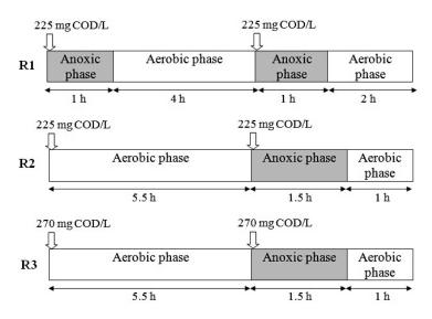
Fig. 1. Cycle configuration of the experimental reactors
