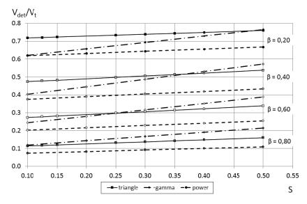
**Fig. 4.** The impact of the hydrograph asymmetry coefficient (S) and the peak flow reduction coefficient on the dimensionless volume of the detention reservoir (V<sub>det</sub>/V<sub>t</sub>) for the inflow hydrographs: triangular, defined by the power function and defined by the gamma distribution
