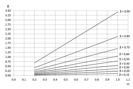
Fig. 2. Effect of hydrograph asymmetry coefficient (ω) and peak flow reduction coefficient (β) on the value of parameter (R) for triangular hydrograph
