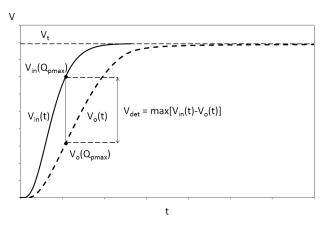
Fig. 1. Diagram depicting methods of calculating the storage reservoir capacity based on: a) inflow and outflow hydrograms, b) inflow and outflow cumulative curves
