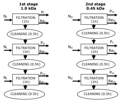
Fig. 2. A block diagram of the conducted experiment featuring the 1<sup>st</sup> and 2<sup>nd</sup> filtration stages. N<sub>I</sub> – feed tank I (effluent water from RAS); N<sub>II</sub> – feed tank II (mixed permeates P<sub>I</sub>, P<sub>II</sub>, P<sub>III</sub> from the 1<sup>st</sup> filtration stage); Re<sub>I-VI</sub> – retentates
