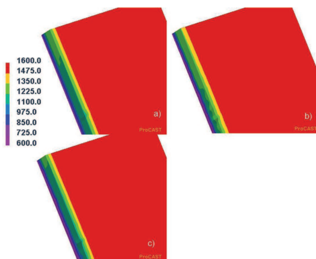
Fig. 5. The temperature distribution (°C) for: a) the reference parameters, b) increased casting speed, c) increased the intensity of cooling
