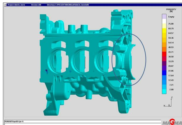
Fig. 13. Porosity measured in 4<sup>th</sup>-bearing area of engine block, die-cast with LSC, top view of bearing [6]
