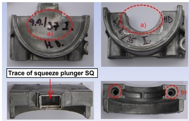
Fig. 3. Different shapes of the bearing area of upper part of old block (with LSC) and new block [3]
