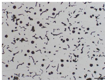
Wall thickness 8mm, 0.013%Mg, 24.9%SGI
