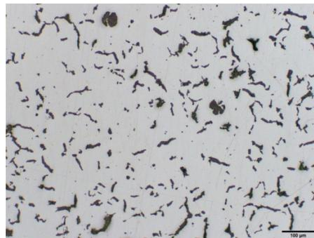
Wall thickness 40mm, 0.013%Mg, 1.5%SGI
