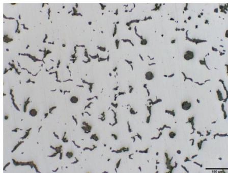
Wall thickness 16mm, 0.013%Mg, 15.2%SGI
