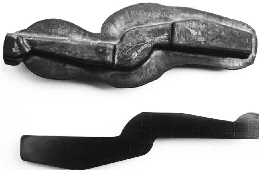
Fig. 5. Forging made in drop forging process and the cut sample used in hardening measurements
