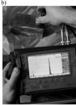
Fig. 2. View of example results of ultrasonic non-destructive testing of bimetallic layered castings: a – lack of joint between the working layer and the bearing part, b – permanent joint between the working layer and the bearing part
