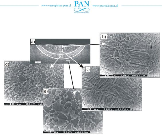
Fig. 3. The microstructure of S355NL steel after remelting with the electric arc: a) heat influence zones on the material, b, c,) the remelted zone - structure: lamellar martensite, d) heat influence zone - structure: martensite ferrite, e) substrate material - structure: pearlite, ferrite
