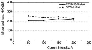
of the tested steels in the function of the current of the electric arc
