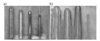
Fig. 1. Steel after remelting with different the current of the electric arc a) X5CrNi18-10, b) S355NL
