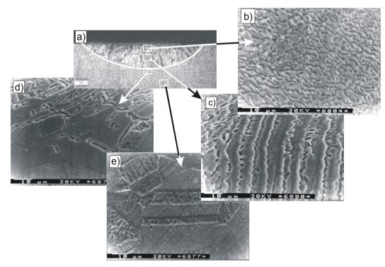
Fig. 4. The microstructure of X5CrNi18-10 steel after remelting with the electric arc: a) heat influence zones on the material, b, c,) remelted zone, d) heat influence zone, e) substrate material - structure: austenite
