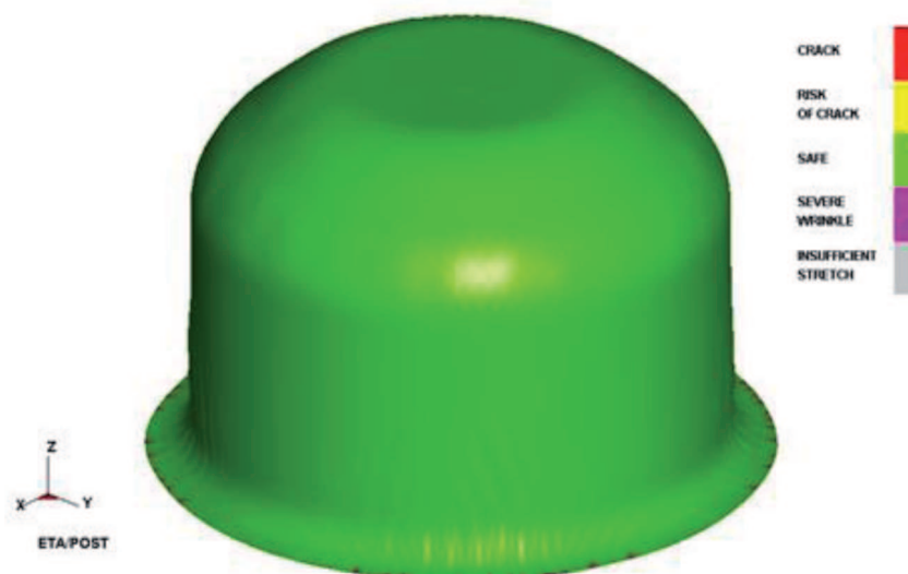
Fig. 10. Final shape of bearing housing
