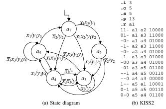
Fig. 1. Example of FSM S<sub>1</sub>.
