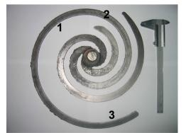
Fig. 5. Photograph of Archimedes spiral and fluidity distance L; 1wall thickness 1 mm, L =200 mm, 2 - wall thickness 2 mm, L =650 mm, 3- wall thickness 3 mm, L =1090 mm
