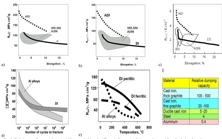
Fig. 1. Relative tensile strength (a,e) yield strength (b) and stiffness indicator (c) fatigue resistance (d) and relative dumping capacity (f); 355, 356, A356 – aluminum alloys. DI – ductile cast iron, ADI – austempered ductile cast iron according to ASTM
