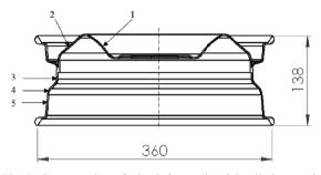
Fig. 9. Cross section of wheel rim made of ductile iron and location of metallographic examinations
