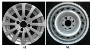
Fig. 8. Wheel rim made of aluminum alloy (Al-Si7Mg) - a), and wheel rim made of ductile iron -b)
