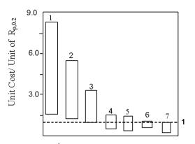
Fig. 2. Unit costs<sup>1</sup> of product essential for obtaining unit yield strength R<sub>p0.2</sub> normalized towards forget steel (up to 1); (1) - aluminum alloys castings, (2) – forged aluminum, (3) – cast steel, (4) – forged steel, (5) - heat treated steel, (6) – ductile iron, (7) – ADI [1]
