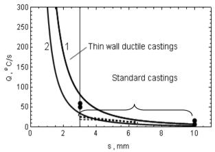
Fig. 3. Influence of wall thickness s and temperature  $T_i$  of liquid metal on the cooling rate of castings: line 1 – prediction for C=3.6%; Si = 2.7%;  $T_i = 1340$  °C, c = 5.95 J/cm<sup>3</sup>a = 0.11 J/(cm<sup>2</sup> s<sup>1/2</sup> °C), line 2 – prediction for C=3.6%; Si = 2.7%; c = 5.95 J/cm<sup>3</sup>,  $T_i = 1450$  °C, a = 0.09 J/(cm<sup>2</sup> s<sup>1/2</sup> °C) [4], points – experimental data [5], lines ----- experimental data [6]
