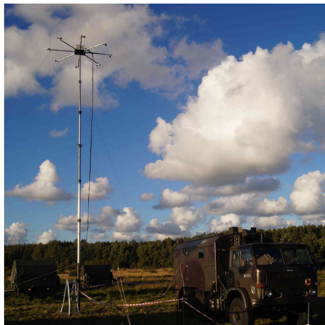
Fig. 7. Deployable mast (12m height) of the PaRaDe system with 8-element antenna array.
