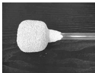
Fig. 2. Ceramic mould used for the permeability testing [13]
