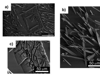
Fig. 4. The block macro-particle (c) and needle-shaped forms (b) of the  $Zn_{16}Ti$  phase
