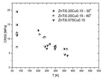
Fig. 7. The CRSS relation to the temperature for two variants of samples orientation. For compare were presented results for Zn-Ti0.075-Cu0.15 single crystals. The anomaly zone was existed only for single crystals with smaller content of titanium
