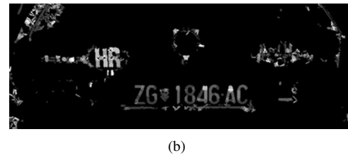
Fig. 4. Stroke width calculation (a – SWT principle, b – SWT image)
