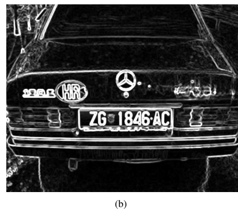
Fig. 6. Application of convolutional operator (a – morphological gradient, b – contrast enhancement)
