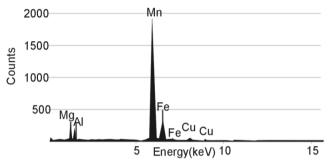
Fig. 8. Local chemical analysis of the precipitates containing Mn, Mg, Al, Cu and Fe in sample 1
