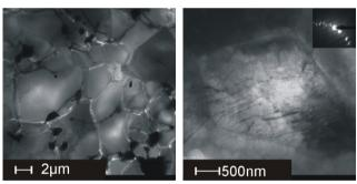
Fig. 6. The microstructure of sample 1 equiaxed grains and slip bands
