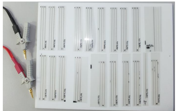
Fig. 2. Cut samples subjected to resistance measurements
