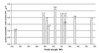
Fig. 6. Mean surface area of κ-phase precipitates in the microstructure of 10 selected BA1055 bronze castings of varying tensile strength
