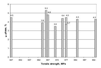
Fig. 5. κ–phase content in the microstructure of 10 selected BA1055 bronze castings of varying tensile strength
