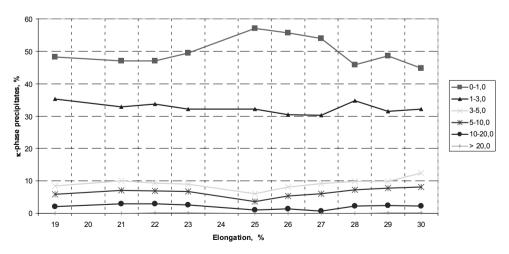
Fig. 8. Elongation of ten BA1055 bronze melts depending on the size and distribution of  $\kappa$ -phase precipitates
