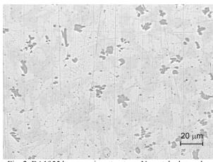
Fig. 2. BA1055 bronze microstructure. Non-etched sample. Visible precipitates of  $\kappa$ -phase
