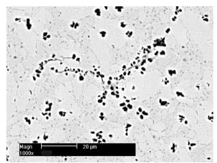
Fig. 10. The shape and location of the κ–phase precipitates in the microstructure of BA1055 bronze castings, (SEM)
