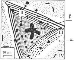
Fig. 1. Shapes of  $\kappa_{I_i}$   $\kappa_{III_i}$   $\kappa_{IV_i}$  phase precipitates in the BA1055 bronze microstructure [7]
