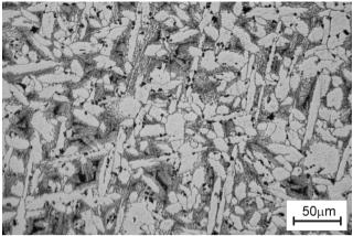
Fig. 3. Microstructure of cast BA1055 bronze; etch. Mi17Cu. The darker κ-phase precipitates at the matrix consisting of α-phase (bright) and eutektoid  $\alpha$ + $\gamma_2$  (grey)
