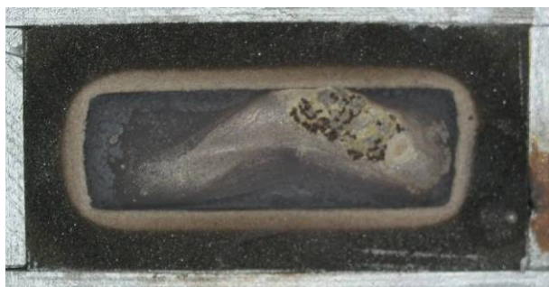
Fig. 3. Effect of the thermal 'self-reclamation' in the immediate vicinity of walls of a moulding sand with an organic binder
