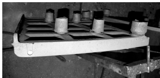
Fig. 6. Plate bent along the short side – variant 3 [4]
