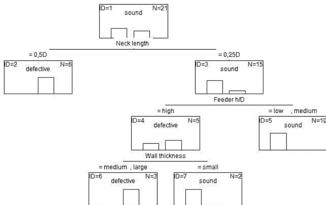
Fig. 8. Classification tree for steel plate-shaped castings with conventional side feeders; two classification results (leaves) with 'sound' class can be seen in the bottom right part of the graph
