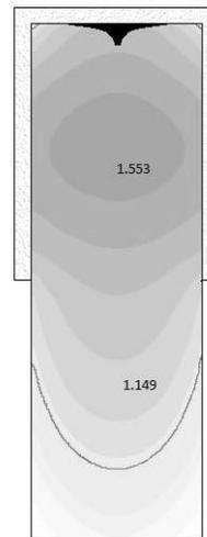
Fig. 2. Simulation results of the cylindrical casting used for calculation of the exothermic sleeves efficiency assumed in NovaCast software; the numbers indicate thermal moduli at the geometry centres of the both halves of the casting: upper (with sleeve) and lower (without sleeve)
