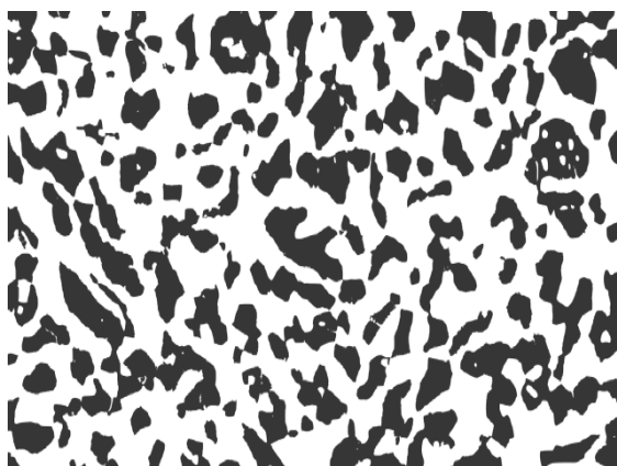
Fig. 6. Metallographic image of the etched duplex steel structure after graphical processing by INSCAPE
