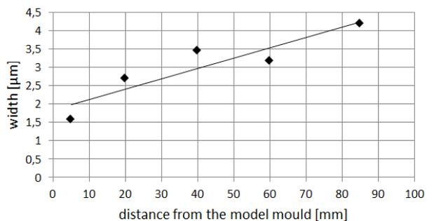
Fig. 5. The average width of carbides on perpendicular sections
