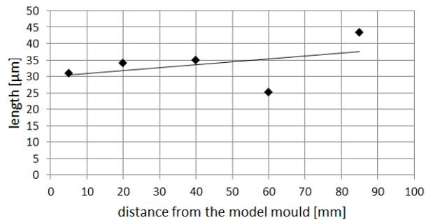
Fig. 4. The average length of carbides on perpendicular sections
