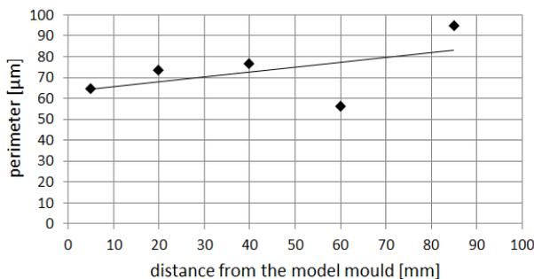
Fig. 3. The average perimeter of carbides on perpendicular sections
