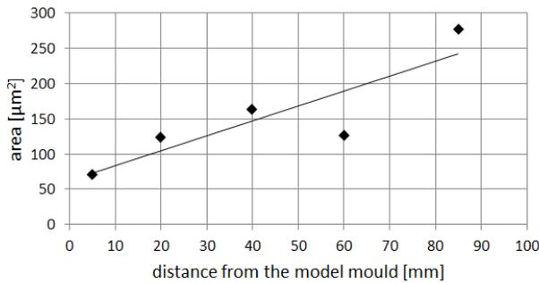
Fig. 2. The average size of carbides on perpendicular sections
