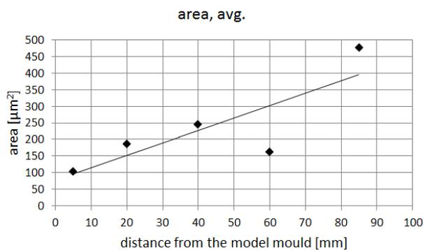
Fig. 7. The average size of carbides on parallel sections
