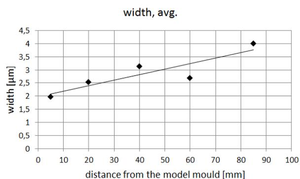
Fig. 10. The average width of carbides on parallel sections
