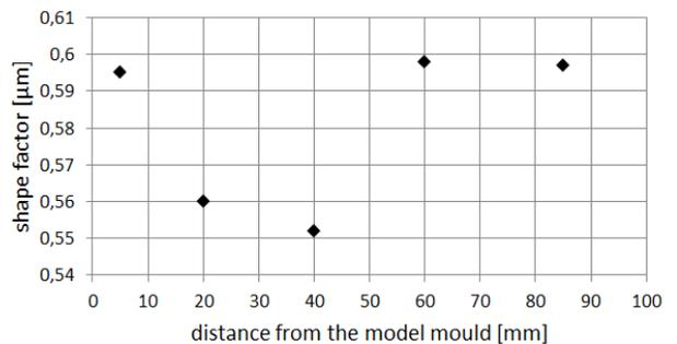
Fig. 6. The average shape factor of carbides on perpendicular sections
