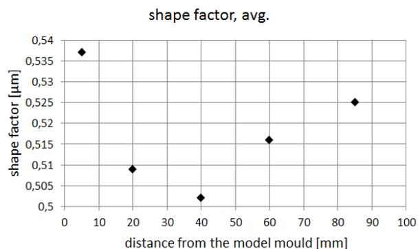
Fig. 11. The average shape factor of carbides on parallel sections
