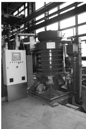
Fig. 3. View of the experimental reclaimer at the background of the reclaim proportioning system into the pneumatic classifier
