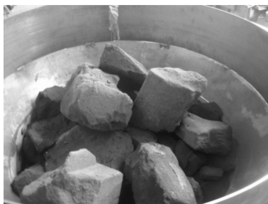
Fig. 5. Agglomerates of used moulding sand with furan resin (on the crushing sieve)
