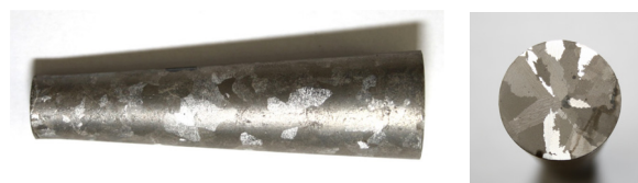
Fig. 6. Macrostructure of side surface and cross-section of test casting (1480°C, white mould, blue filter)
