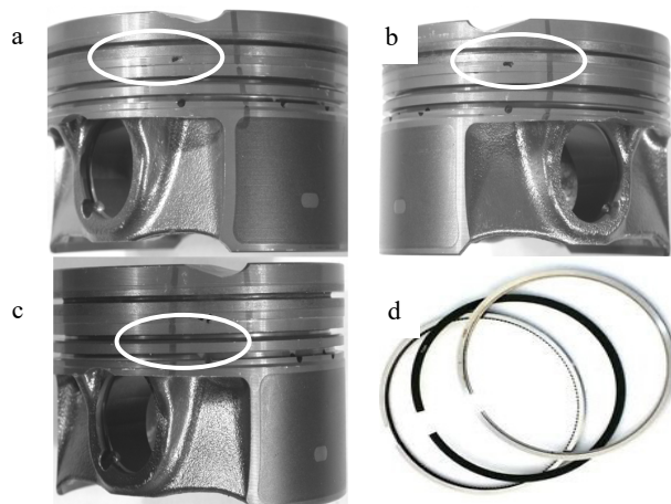
Fig. 1. Shrinkage cavity on the connection place of „alphin” ring with the piston (a-c), piston's rings (d)
