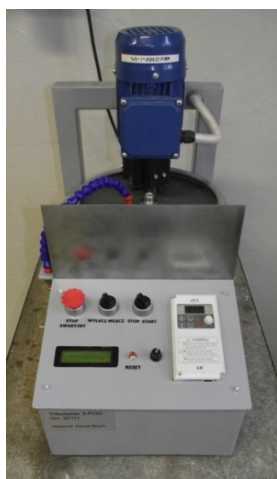
Fig. 2. Scheme and picture of Tribotester 3-POD device
