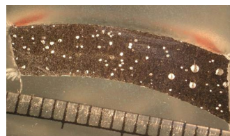
Fig. 2. Fracture through casting with gas porosity
