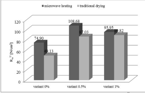
Fig. 2. Effect of water addition and hardening method on tensile strength  $R_m^{\cup}$
