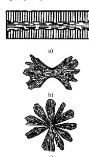
Fig. 9. The changes scheme during solidification of the eutectic with increasing undercooling [16]
