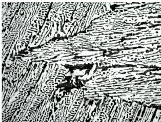
Fig. 2. Two types of cementite plates: longitudinally growing in middle set; and growing perpendicularly - in honeycomb eutectics. Own research, LM x 200
