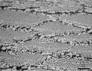
Fig. 4. Structure of eutectic pyramid in ledeburite, LM
