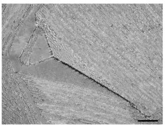
Fig. 6. Structure of eutectic pyramid of researched sample, light microscopy
