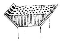
Fig. 3. The model forming of eutectic pyramid [14]
