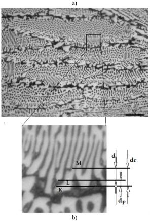
Fig. 13. The distance in researched sample of ledeburite eutectic, a) light microscope x500,
