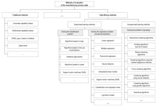
Fig. 3. Classification of methods of evaluation of the manufacturing process state (own work on the basis of [8–10]).
