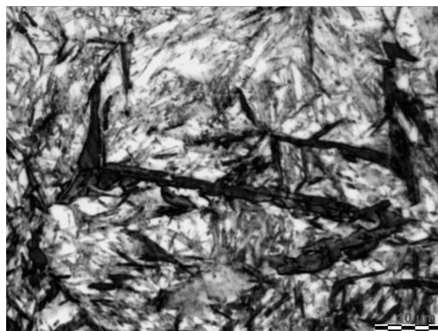
Fig. 7. Observation of microstructure details with visible lower bainite accelerated by small amounts of prior athermal martensite after austempering with isothermal transformation at 160°C during 3 min., etching with nital
