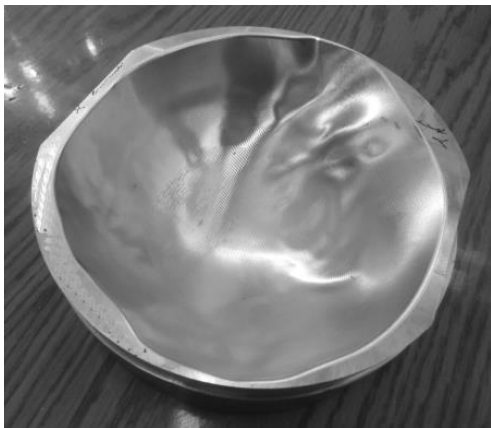
Fig. 7. Die-block for mould-incremental sheet forming.
